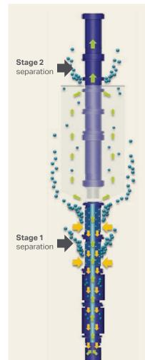
An operator in Colombia wanted to reactivate a gassy, depleted well in a field where artificial lift methods were deemed unsuitable due to high Gas to Liquid Ratio (GLR). Alkhorayef designed a shrouded ESP with two stages of gas separation that simultaneously increased gas and oil production.
