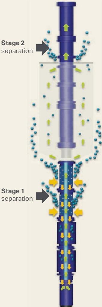
An operator in Colombia wanted to reactivate a gassy, depleted well in a field where artificial lift methods were deemed unsuitable due to high Gas to Liquid Ratio (GLR). Alkhorayef designed a shrouded ESP with two stages of gas separation that simultaneously increased gas and oil production.
