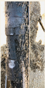
Evidence of the Reservoir Damage on the Pulled ESP
